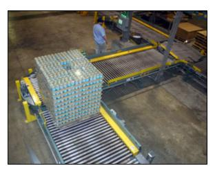
Many operations utilize pallet or slip-sheet to convey bulked material, whether in manufacturing, work in process, to feed a palletizer, or in shipping areas.
